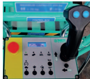
Control panel on the platform with capacitive buttons: simplicity and safety of use
